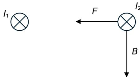
where  $B$  is the magnetic field created by the wire on the left at the position of the wire on the right. Comparing  $F = \frac{\mu_0 I_1 I_2 L}{2\pi r}$  to  $F = BI_2L$  we see that  $B = \frac{\mu_0 I_1}{2\pi r}$  i.e. the magnetic field created by a long straight wire carrying current  $I$  at a distance  $r$  from the wire is
